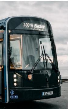
Oval-shaped glass with curved front and rear parts increases the aerodynamics, visibility of the bus, gives a more spacious feel.
