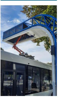
500kW ultra-fast battery charging at the end of the route allows you to charge the batteries in less than 8 minutes.
